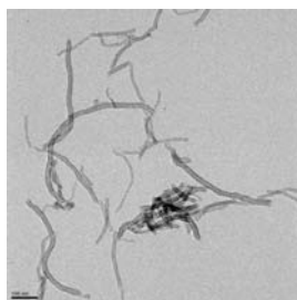
(a) High resolution TEM image of pristine MWNT. The MWNTs consist of a high number of parallel carbon walls, which are undamaged. The external diameter is approximately 22 nm while the inner diameter of the CNT is only 5 nm.
